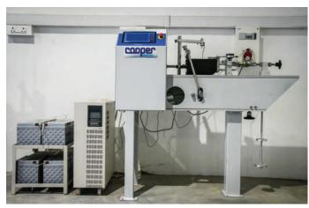
Automated direct shear apparatus
