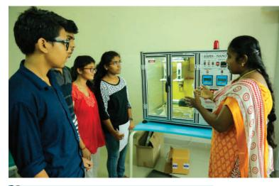
The instructor explaining about the functioning of Electrospinning Apparatus
