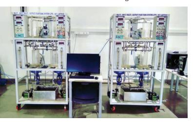
MIMO 4-Tanks System at the Advanced EE Lab
